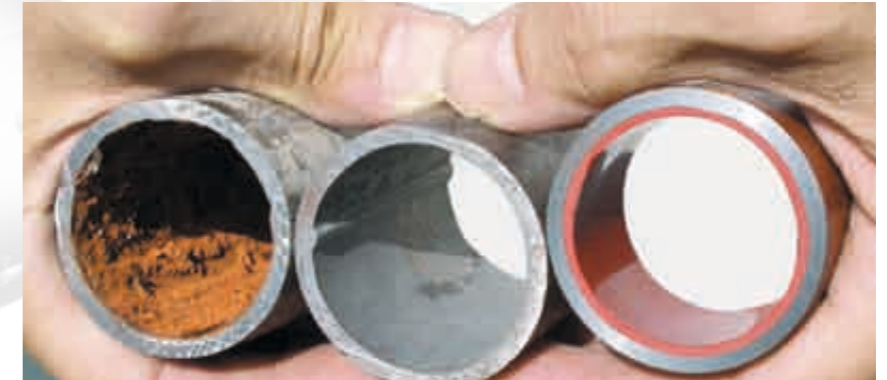
2) Restoration of pipework by the Promotec-system; corroded, cleaned and coated pipes
