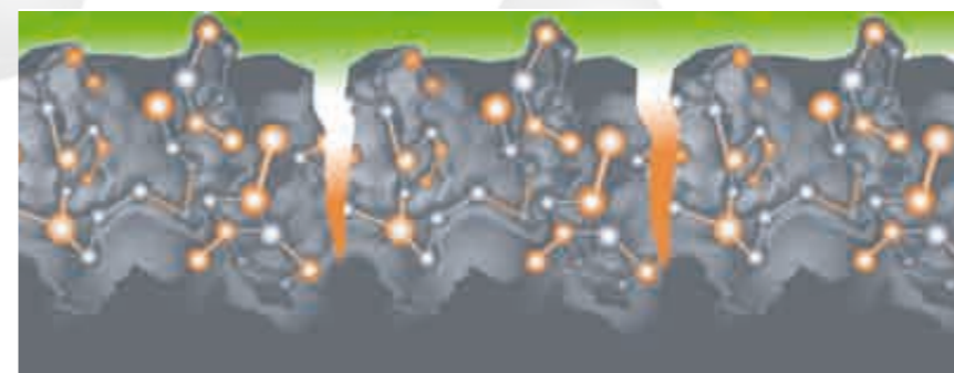
Picture: Effect of our tank lining product. As soon as micro cracks occur in the coating, the special biocide crystals burst and unfold their effect within the whole crack. The SRB are killed before their settlement. The existing depot effect causes a long-lasting biocidal corrosion protection without localized erosion.
