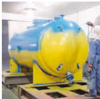
5) Drinking water tank, internal and external coating
