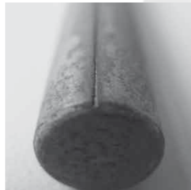
3) Coating without biocide After a month-long test the pickled test rod shows deep biocorrosion. (depth of corrosion cavity 150-200 µm)
